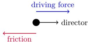
FIG. 1. A balance of the driving force in the direction defined by the ‘director’ unit vector and the friction due to the Langevin thermostat results in a constant terminal velocity.
