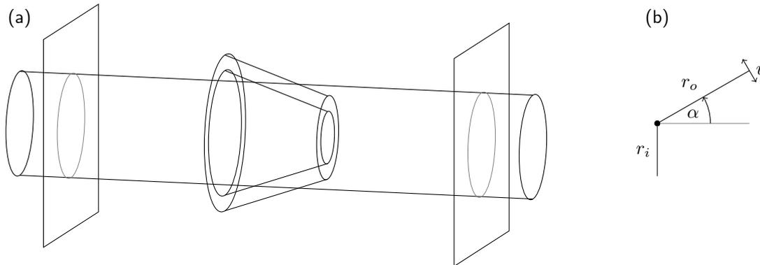
FIG. 4. (a) Sketch of the rectifying geometry which we simulate for this tutorial. (b) The geometry of the `HollowCone` constraint and `LBBoundary`. The figure is cylindrically symmetric about the x-axis. The size of the pore opening is determined by  $r_i$ , the length of the cone by  $r_o$  and the opening angle by  $\alpha$ . Finally, the pore is given a width using the parameter  $w$ .
