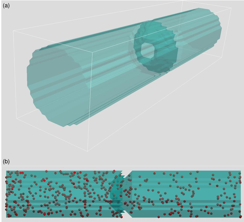
FIG. 5. (a) Snapshot of the rectifying geometry, as visualized with ParaView. (b) Final state for the system with 500 particles and  $vel=5.0$ . Note that there are more particles in the left-hand chamber, due to the rectification.
